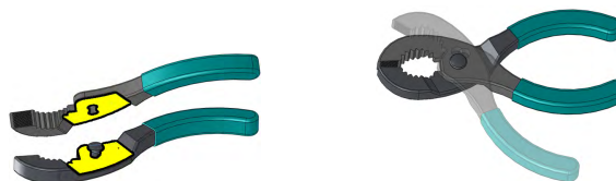
(a) A plane-plane coincidence constraint used in the design. (b) Design intent includes rotation.
